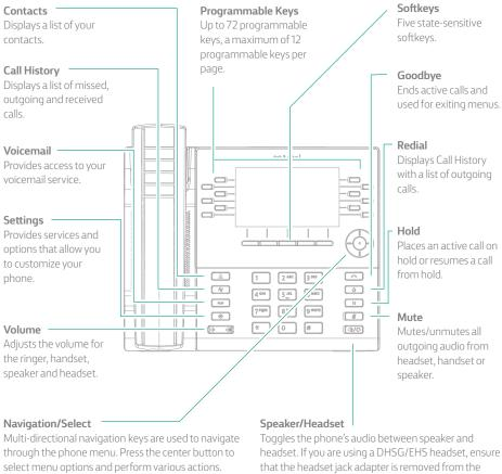
On the Home screen, the left and right navigation keys can be used to access the additional pages of programmable keys.
